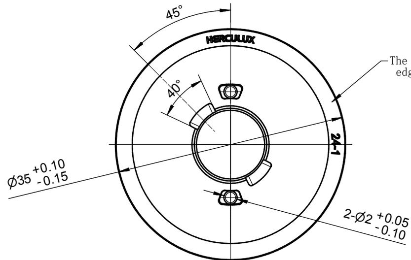
The bottom surface of mounting edge is frosted surface
